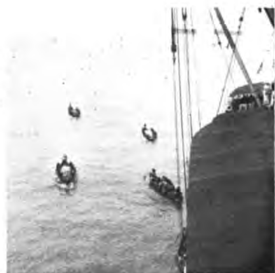
Accra, Gold Coast (Ghana) Cargo is lightered to/from ships offshore in 'surf boats' carrying about 2 tons each trip. These boats have a free-board of only a few inches. They are staffed by 10 paddlers and 1 helmsman. Men work scantily clad - the paddles of various boats are made up in various colors and designs to drive away the evil spirits. Pix by A. R. Gilmore on the African Pilot - 1954.
